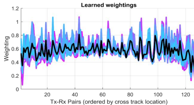
Figure 31: Multiple examples of learned Tx-Rx pair weightings. The average is also plotted as the solid black line. Notice the consistent pattern over many of the learned responses, this implies that some antennas are not as useful in accentuating the target-like radar responses. There is also an overall trend of higher weighting in the center of the array and less weight towards the outside elements of the array.
