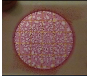
E. COLI WATER SAMPLE TEST DISK WITH A SAMPLE OF PARTICULARLY BAD WATER
