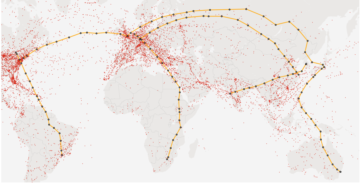
Figure 2.3: Using in-flight aircraft as network hops. This snapshot from July 11, 13:49 UTC shows 11,082 in-flight aircraft as well as the paths between a few major cities through them.
