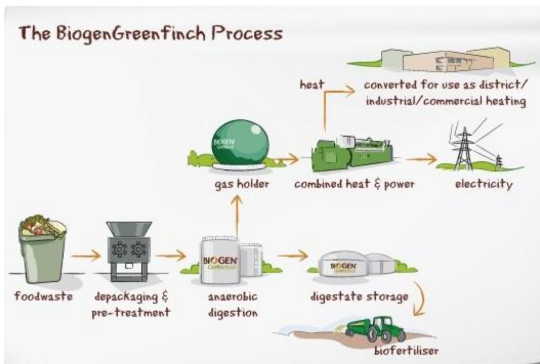
Figure 10: Anaerobic Digestion Process
