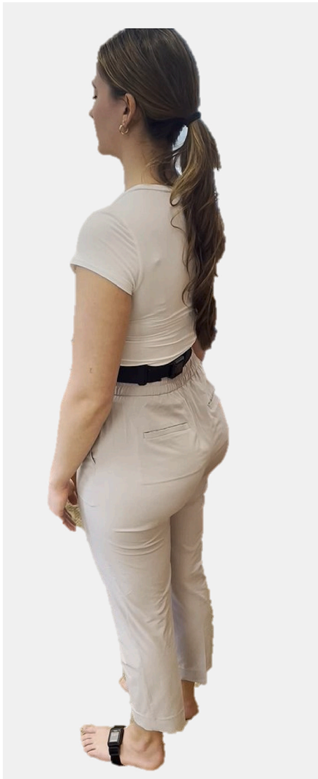
Fig. 1. OPAL IMU-Based Sensors for Gait and Balance Tests: one pelvic sensor and two foot sensors.
