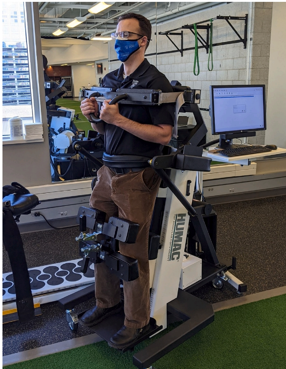
Fig. 2. Trunk Sensorimotor Testing. The monitor was later positioned in front of the subject during actual testing to provide visual cues and feedback for visual-motor reaction time and force steadiness testing, respectively.
