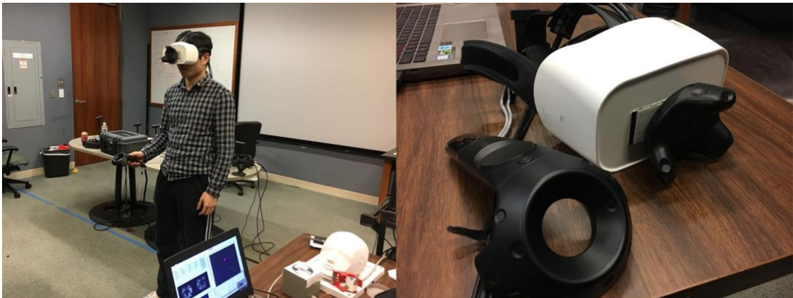
Figure 4: Experiment participant and FOVE headset (with an HTC Vive tracker) and HTC Vive controller.
