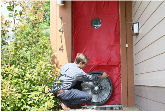
Fig. 4 Blower door test (Source: Clinton Climate Initiative)
