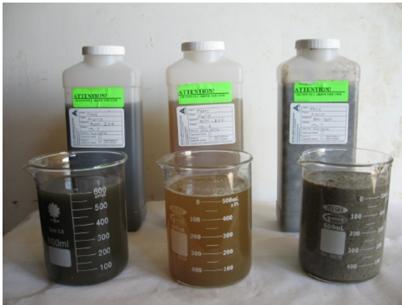
Figure 13. Influent – Effluent – Separated Solids
