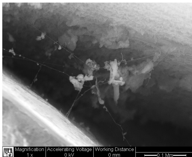
Figure 19: Thin polymers connecting silica gel to cube surface, seen in 200 ppm Si ion concentration pH 2.5 solution after 3 weeks aging
