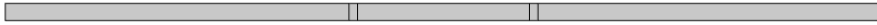
FIGURE 8.2: Fabry-Pérot cavity: (left) vacuum domain; (middle left) dielectric wall; (center) cavity domain; (middle right) second dielectric wall; (right) second vacuum domain. The pump beam enters from the left and travels to the right.
