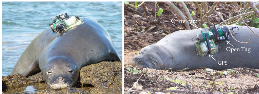
Figure 14: Photo of the instrument package attached to a Hawaiian monk seal
