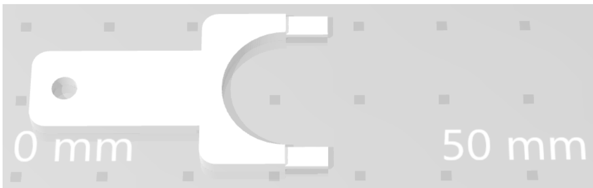
Figure 7: Render of a 3D-printed window holder. Two holders, one for each side, are mounted to form an imaging jig which holds the window stable and reduces motion artifacts caused by respiration.
