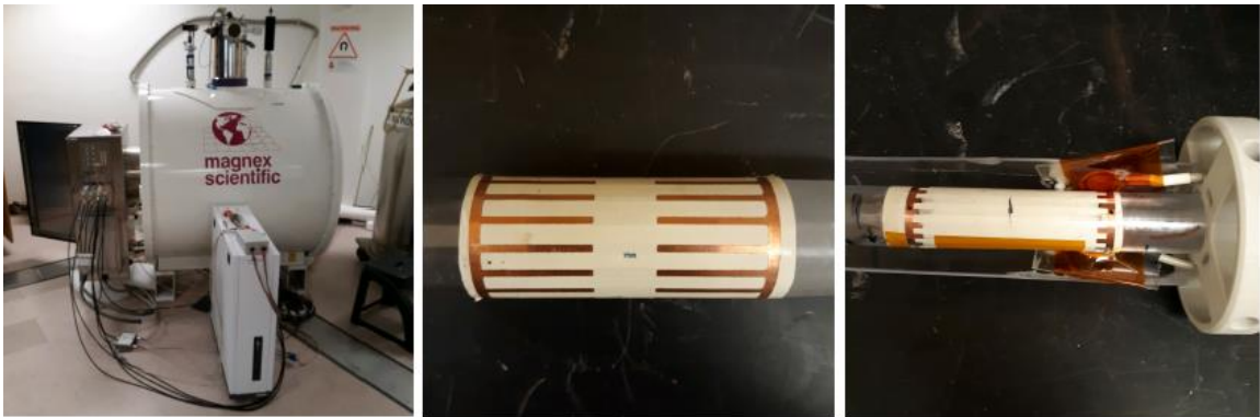
Figure 25: DT-MRI acquisition setup for whole mouse tractography. Left – GE 7T research MRI unit. Center – inverted custom birdcage coil showing the interior material patterning. Right – Homemade low pass birdcage coil using a custom dielectric, mounted with pickups. The mouse is placed in the center of the coil, and the coil is centered in the magnet chamber for optimal field exposure.
