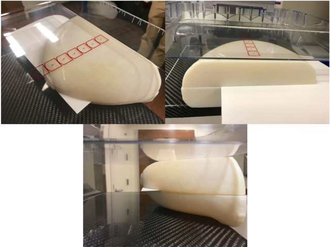
Figure 3. Photographs of contrast-detail insert sandwiched in mid-depth of physical breast phantom, which is positioned and compressed like a real patient on a Hologic DBT system.
