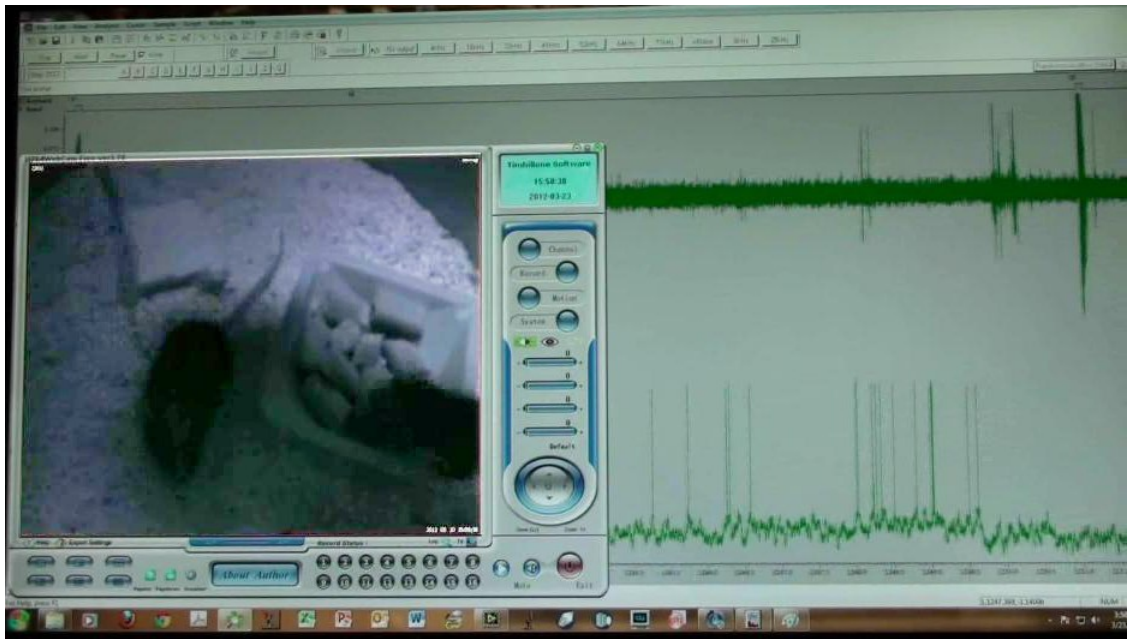
Figure 15: In vivo intracellular recording with a Yaris system (microdrive + the mini-headstage) from a freely behaving mouse with another mouse. Left: video monitoring via inside camera, left mouse is the subject. Right: real-time intracellular signal (lower green trace).
