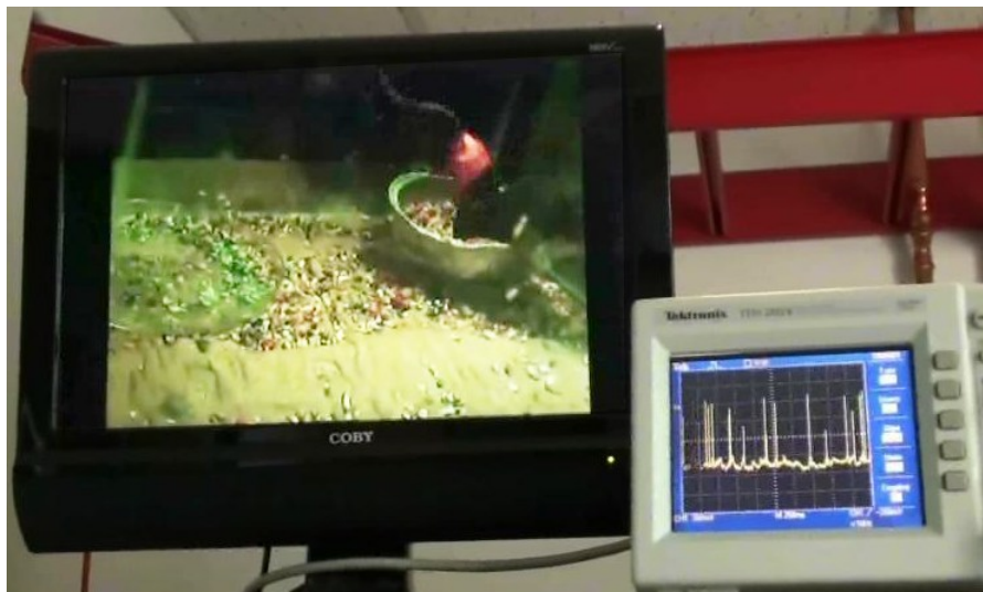
Figure 14: In vivo intracellular recording with a Yaris system (microdrive + the mini-headstage) from a freely behaving zebra finch. Left: video monitoring via an inside camera; the bird is pecking a seed tray. Right: real-time intracellular signal on an oscilloscop
