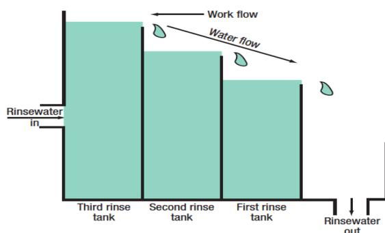
Figure 15: counter-current rinsing system<sup>51</sup>
