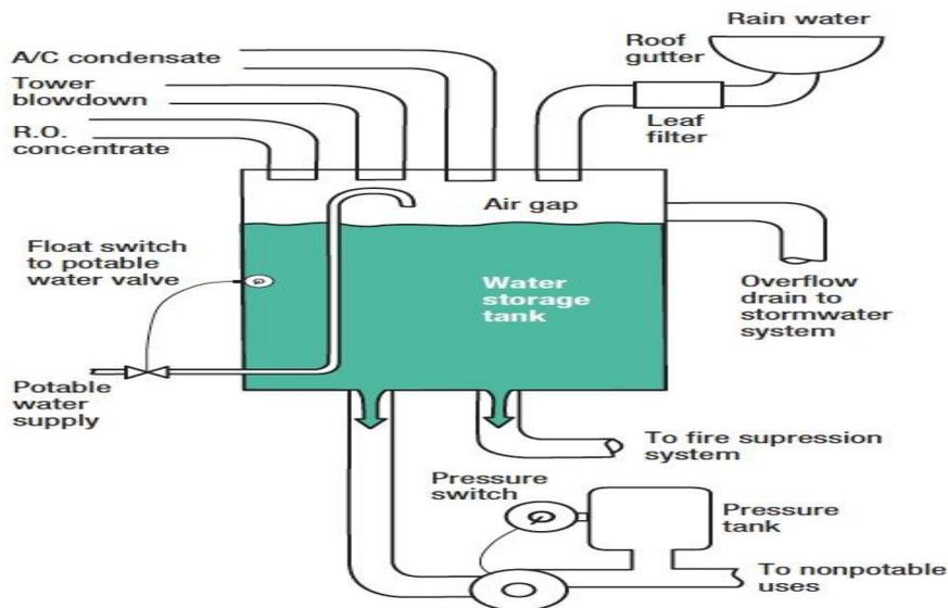
Figure 11: non-potable water collection and reuse<sup>45</sup>
