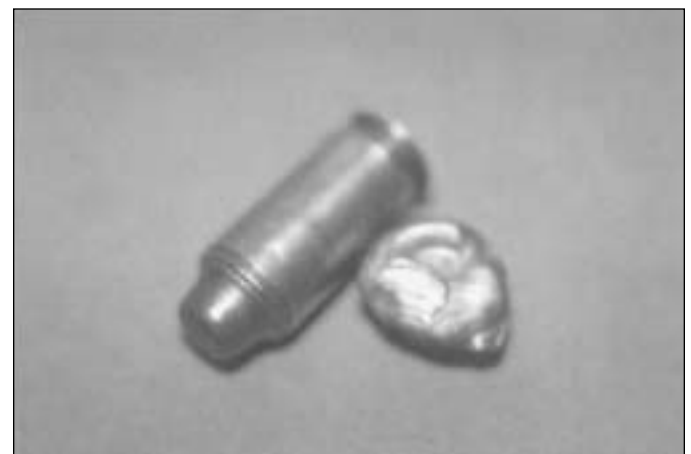
Figure 3. Projectile construction of unjacketed or partially jacketed lead deforms on impact with higher-density media such as human tissue. This results in increased cross-sectional diameter, which in turn increases the potential for both crush injuries (permanent cavity–anatomic factor) and stretch injuries (temporary cavity–energy transfer factor) depending on other projectile characteristics.
