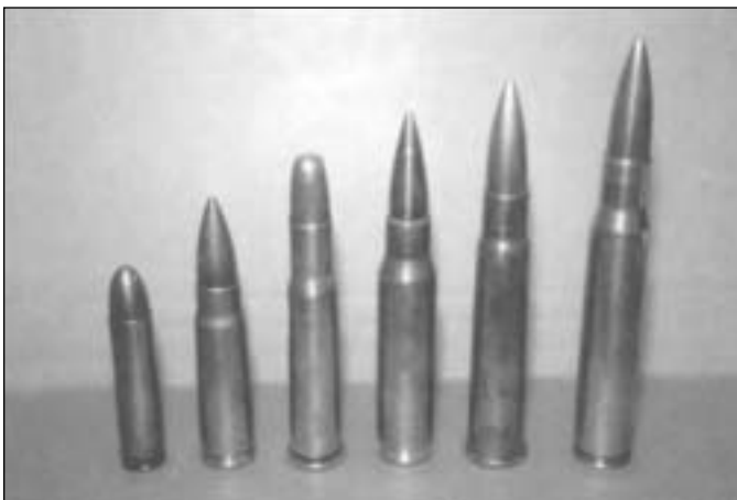
Figure 2a. These projectiles are, from left to right, .30 M-1 carbine, 7.62x39 mm, .30-30 Winchester, 7.62x51 mm NATO, .303 enfield, .30-06 M-1. Although significantly different in multiple parameters, these projectiles all have approximately the same caliber, emphasizing the point that caliber alone is of little value in estimating wounding severity.
