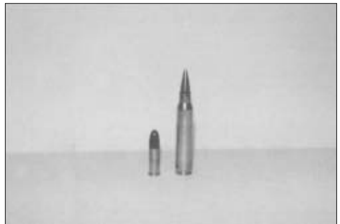
Figure 2b. These projectiles are, from left to right, .22 rimfire (used in handguns and rifles) and 5.56 mm (.223) M-16. They are of similar caliber but are otherwise significantly different. Again, caliber alone is a poor determinant of wounding potential.
