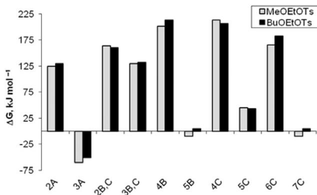
Fig. 7. Comparison of the Gibbs free energy for the MeOEtOTs and nBuOEtOTs systems calculated at M06-2X/6-311++G(2d,p)//M06-2X/6-31+G(d) DFT level for the species associated with the mechanisms given in Fig. 5. Compression and ionic pair effects were taken into account where appropriate (see text). Actual energy values are listed in Supplementary Information.
