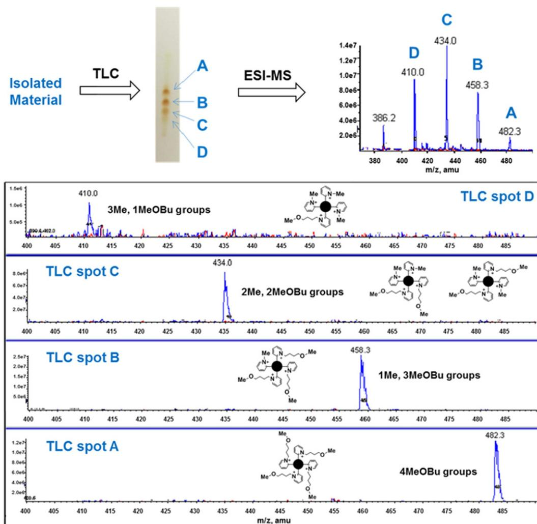
**Fig. 2.** TLC plate and ESI-MS analyses of both the crude mixture and the materials recovered from TLC spots of the “MeOBu/3-Py” system, which was initially thought to yield MnTMOBu-3-PyP<sup>5+</sup>. TLC-SiO<sub>2</sub> was carried out in 1:1:8 = saturated KNO<sub>3(aq)</sub>:H<sub>2</sub>O:CH<sub>3</sub>CN system. ESI-MS peaks in the  $m/z$  370–500 region correspond to ion-pairs ( $\text{MnP}^{5+} + 2\text{HFBA}^{-}$ )<sup>3+</sup>/3.
