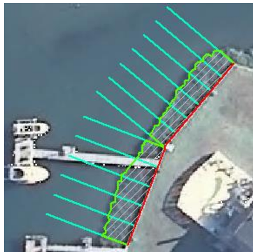
Figure 3: Image of two bulkhead sites in 2013 with bulkhead delineation in red, transects in blue, and the waterward marsh edge in green.
