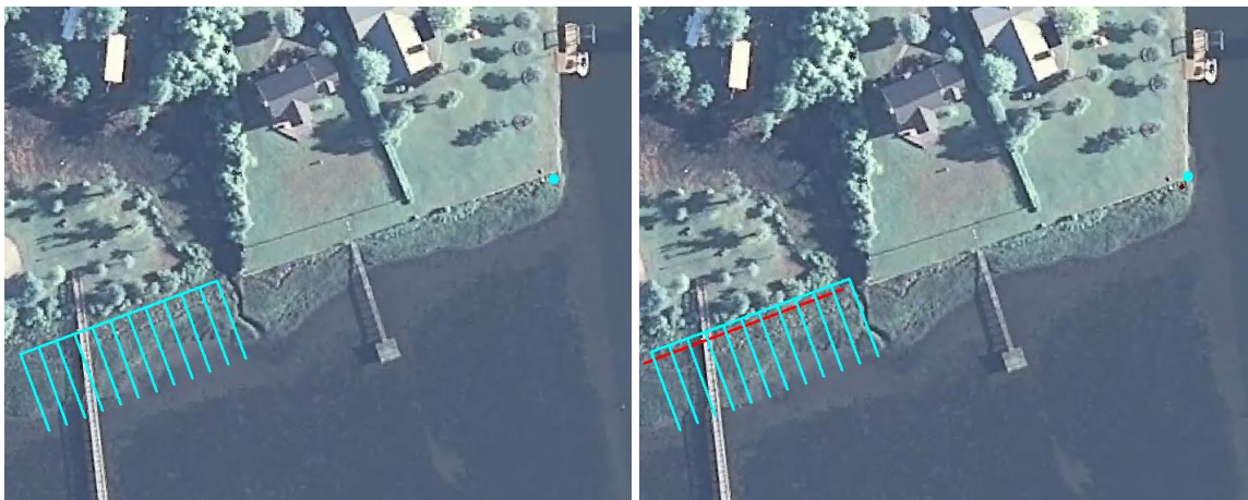
Figure 8: Left image depicts the locations of control site line, transects, and reference point (all in blue), where reference point is offset from corner of the bulkhead. Right image shows result of shifting the site line and transects simultaneously with the reference point, now located at the corner of the bulkhead used as the reference location (red line indicates location of 1981 control site line, blue line is 2013 location).
