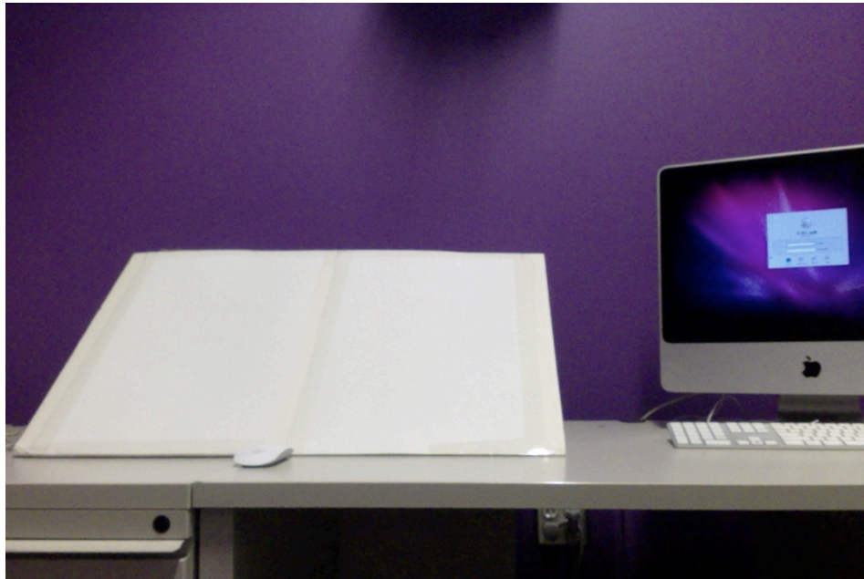
Figure 2: Apparatus used for Study 2. Participants used a cordless mouse to move up a ramp and toward their targeted stimulus of interest. Following trial conclusion, they moved the mouse to the bottom to begin the next trial. Keypresses were generated using the index finger of their dominant hand on the keyboard.
