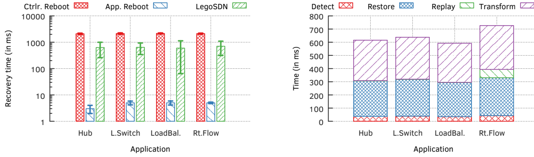
(a) Median recovery time of different techniques: LegoSDN is slower than App. Reboot, but significantly faster than Ctrlr. Reboot.
