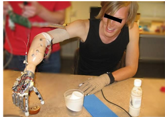
Fig. 1 Amputee reaching an object wearing SmartHand. The unnatural reaching posture of the arm caused by the lack of the 3 degrees of freedom of the wrist/forearm is clear from this picture.
