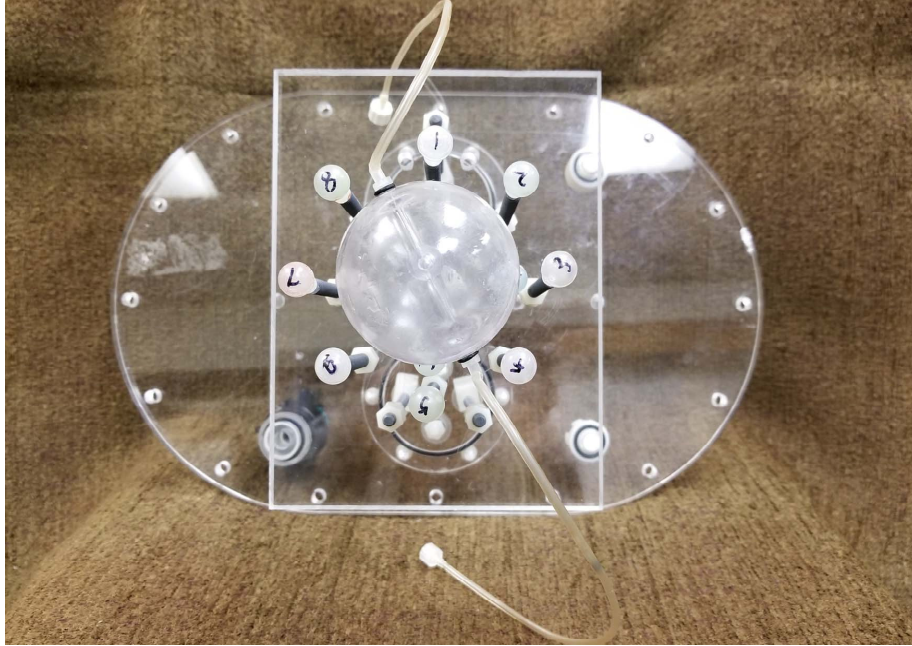
FIGURE 2.1: The bladder insert was vertically and horizontally centered on a perpendicular insert, twelve lesions were also symmetrically placed (only 8 spheres could be seen above).
