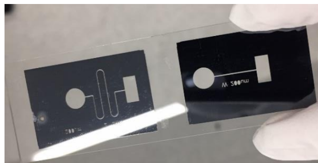
Figure 26: Photograph of microfluidic chip in silicon after it has been bonded to glass using anodic bonding.
