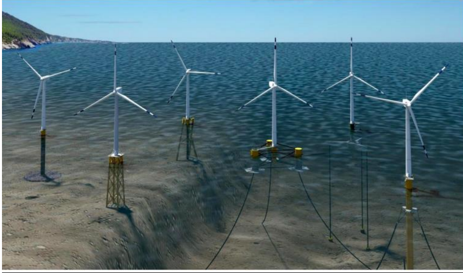
Figure 6: Different offshore foundation types. Left to right: monopile, jacket, twisted tripod, floating semi-submersible, floating tension leg platform, and floating spar. (Credit: Josh Bauer/National Renewable Energy Laboratory)
