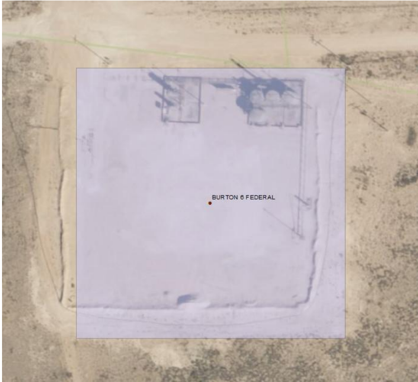
Figure 4: The Burton 6 Federal P&A site shows the approximation of the generated spatial buffer in relation to a plugged and abandoned well site. It should be noted that the imagery is from 2015 while the plug and abandonment activity occurred in 2019.
