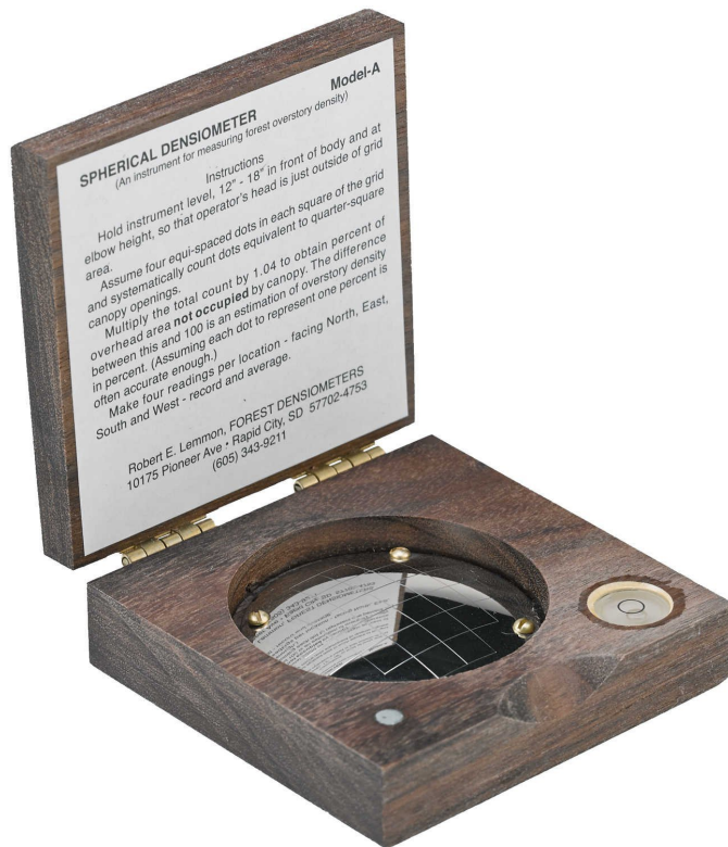
Figure 1 - Image of a Spherical Densiometer 1
