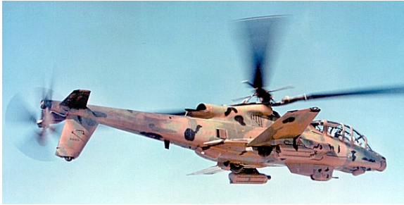
FIGURE 1.2: Cheyenne helicopter, which uses a lifting wing to offload the rotor in forward flight [24].
