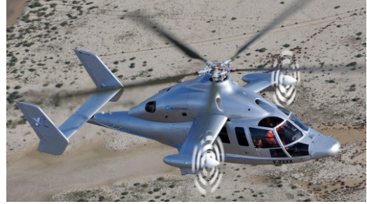
FIGURE 1.3: Eurocopter X3 compound helicopter, which uses a lifting wing with two propellers for auxilliary propulsion [34].
