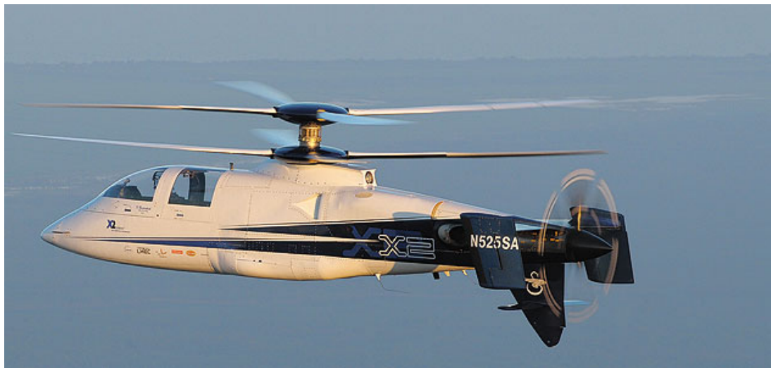
FIGURE 1.4: Sikorsky X2 technology demonstrator, which uses a coaxial rotor and a pusher propeller [35].
