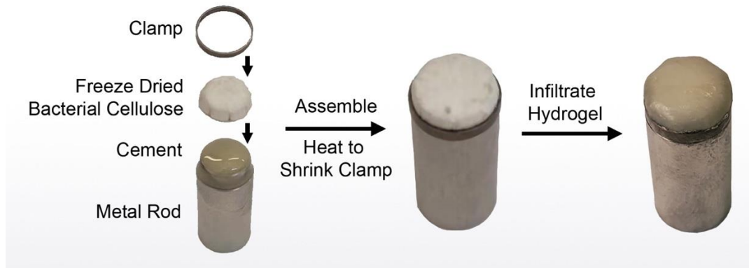
Figure 21: Overview of the method for attaching a hydrogel to a metallic pin with a shape memory alloy clamp.
