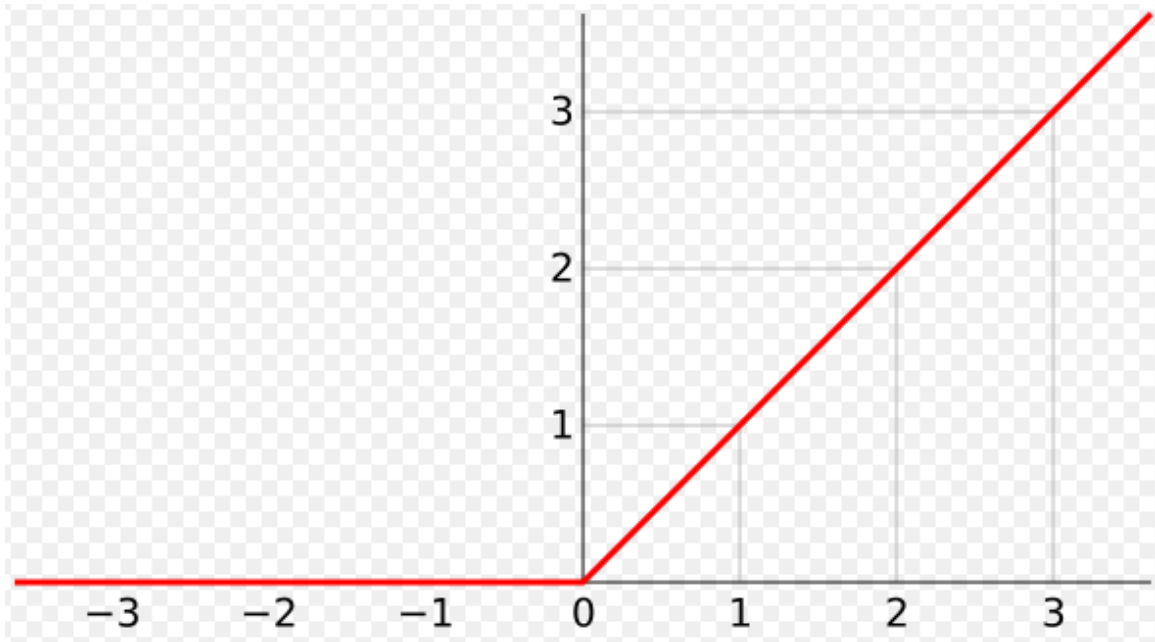
Figure 9 The graph of ReLU function. It is a half linear function. All the input values which is smaller than 0 are set to be 0 and the values greater than 0 remains.
