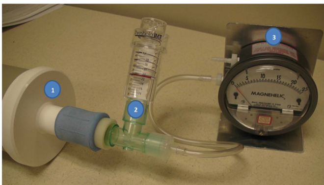
Fig. 1. RMT device calibration methodology. Accomplished using a 3-way gas pressure circuit comprising 1) an air delivery system to introduce positive or negative pressure, 2) the inspiratory or expiratory RMT device being calibrated, and 3) a differential atmospheric pressure gauge.
