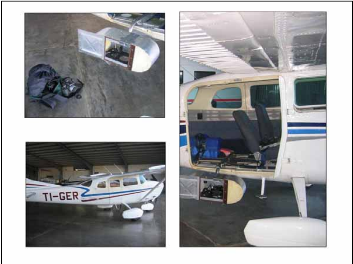
Figure 3: Digital camera platform and airplane used in aerial surveys
