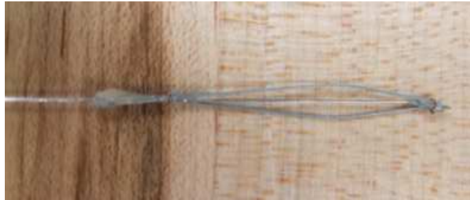
Figure 14: Third iteration prototype, Prototype C. Nitinol wires are fixed to the main nitinol wire using super glue and copper wire.
