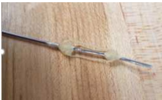
Figure 13: Second iteration prototype, Prototype B. PEEK wires are fixed to the stainless-steel wire using super glue.
