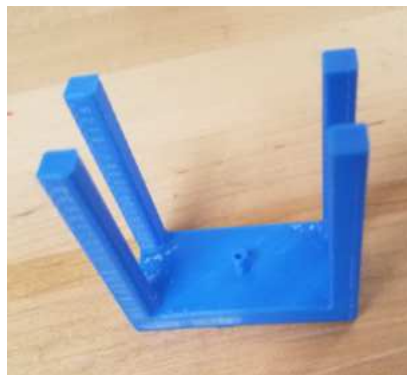
Figure 19: 3D-printed component for fixing porcine artery in Experiment A.
