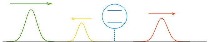
FIG. 4. (Color online) Waveguide setup considered here, where a qubit is side-coupled in a two-terminal geometry to a photonic waveguide. Transport properties are described by scattering processes depicted by a set of ingoing and outgoing wavepackets.
