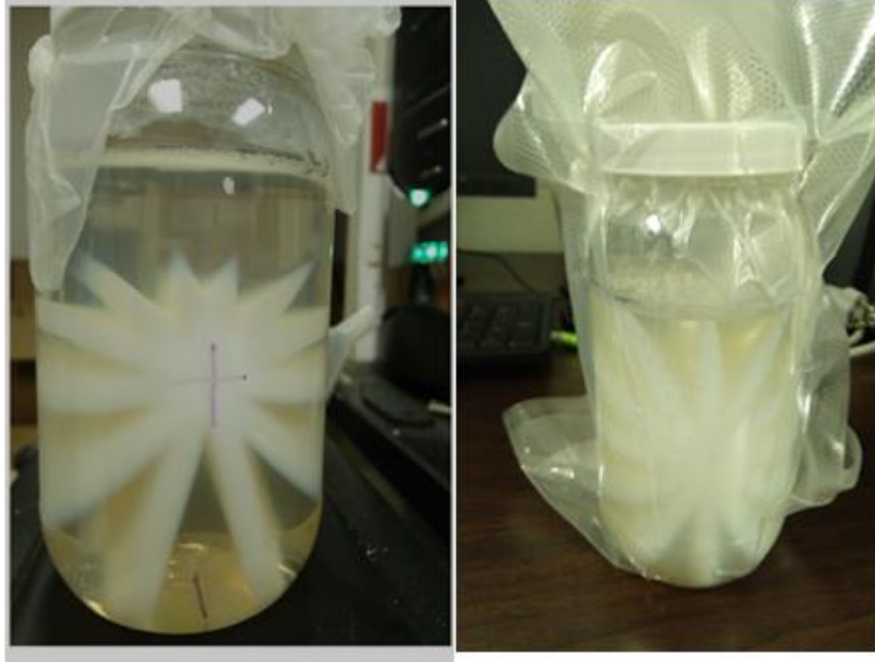
Figure 6: Star shot for Couch rotation (Oxygen and non-oxygen contamination effect)
