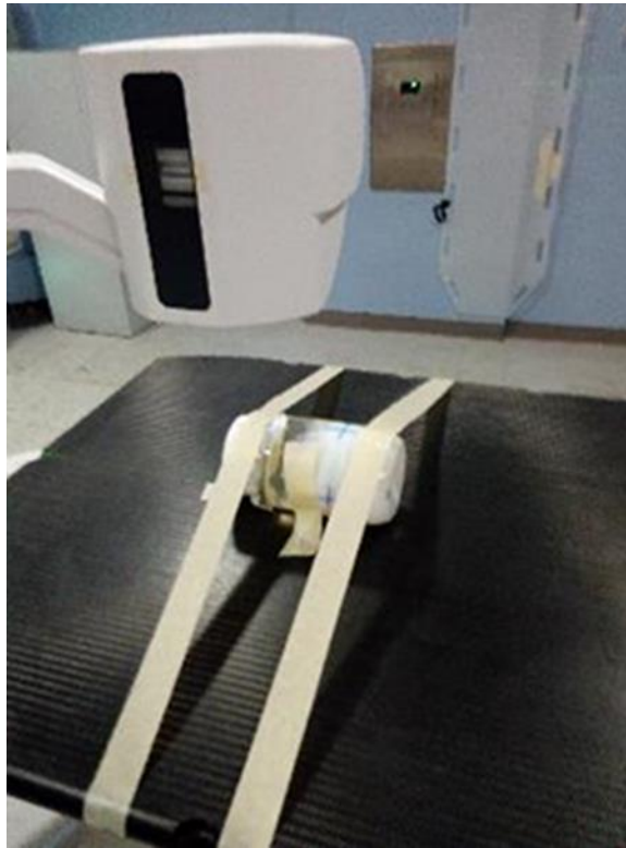
Figure 28: CBCT-D set up of the gel for all-star shots
