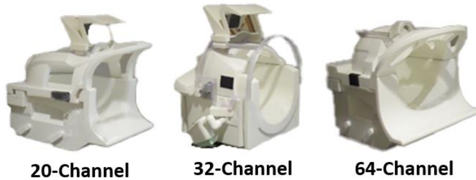
Figure 1.6: Photos of RF receive head coil arrays with increased coil density (i.e., more coil elements placed close to the imaging field of view) 1 .
