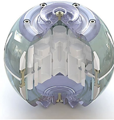
Figure 3.1: Depiction of the Diffusion Standard Model 128[1] phantom used to study the effects of eddy current and EPI distortions.
