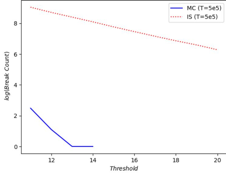
FIGURE 5.1: Comparison of the number of break events for Monte Carlo and importance sampling methods in 500,000 trials, for  $f = 10 \cdot \mathbf{1}$ . In the IS algorithm, we use  $c = 1$ .
