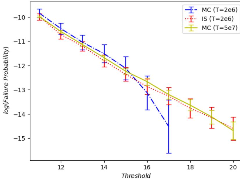
FIGURE 3.3: A comparison of the two MC estimates, and the IS estimate of  $p(b)$  for various  $b$  values in the case of a uniform  $f$ . The IS algorithm is more accurate than MC across all threshold values and is able to generate estimates for a larger range of threshold values as well.
