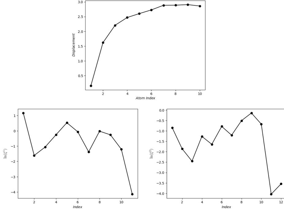
FIGURE 4.2: Solutions to (1.11) exhibiting a break with  $b = 20$ ,  $\epsilon = .1$ , and  $f = 10 \cdot \mathbf{1}$ . The top row depicts the displacement field, while the bottom row shows the log of the  $\xi$  coefficients. In this example, the break occurs at the right edge of the atom chain, between atom 10 and the “ghost atom” at index 11.
