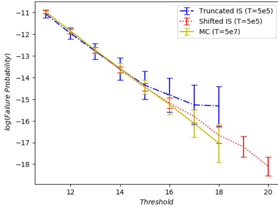
FIGURE 5.9: Comparison of IS methods using shifted and truncated Gaussian distributions for  $Q$ .
