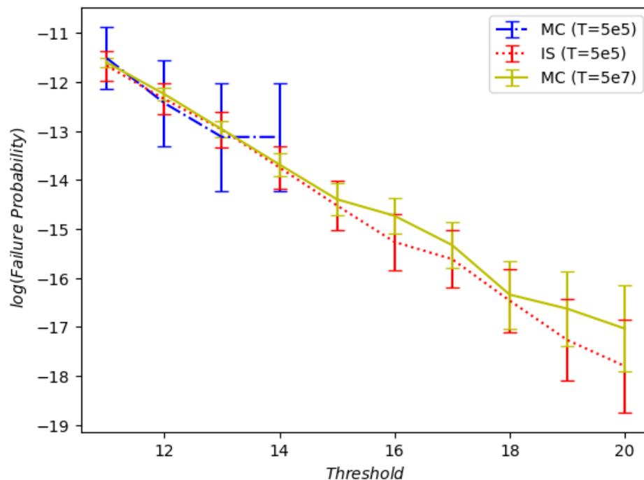
FIGURE 5.4: A comparison of the two MC estimates, and the IS estimate of  $p(b)$  for various  $b$  values, in the case  $f = \frac{5}{\epsilon}e_6$ .
