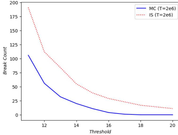
FIGURE 3.1: Comparison of the number of failure events observed from Monte Carlo and our importance sampling algorithm for a single run of 2 million trials and a uniform force  $f = \mathbf{1}$ .
