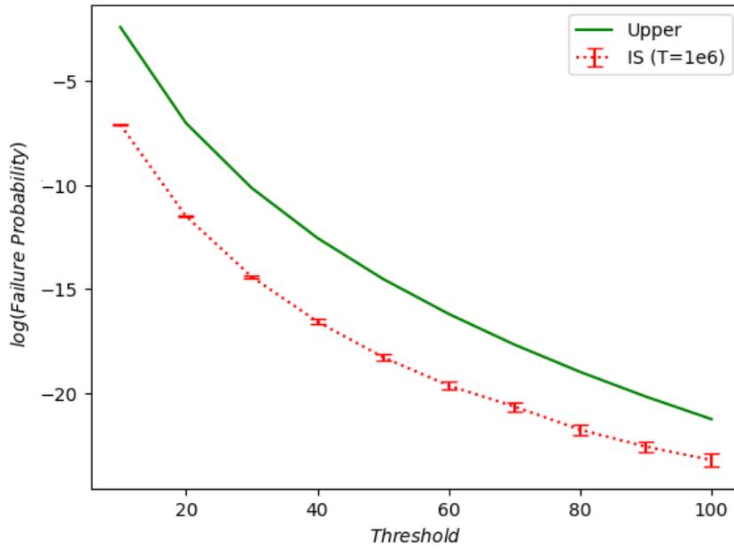
FIGURE 3.5: Comparison of the upper bound in (2.3.6) and numerical calculation of  $p(b)$  for  $b$  values ranging from 10 to 100.
