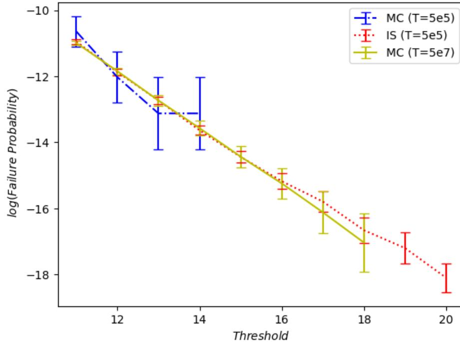
FIGURE 5.3: A comparison of the two MC estimates, and the IS estimate of  $p(b)$  for various  $b$  values, in the case  $f = 10 \cdot \mathbf{1}$ .
