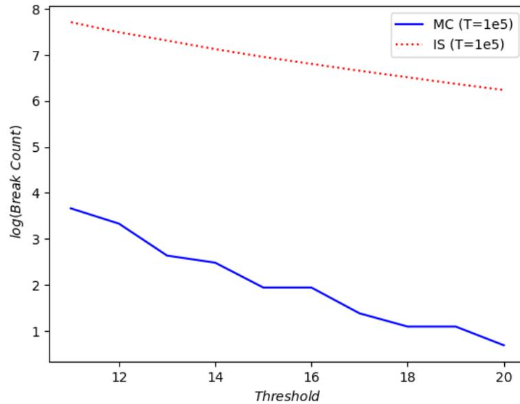
FIGURE 3.2: Comparison of the number of failure events observed from Monte Carlo and our importance sampling algorithm for 100,000 trials and a localized force  $f = \frac{1}{\epsilon} e_6$ .
