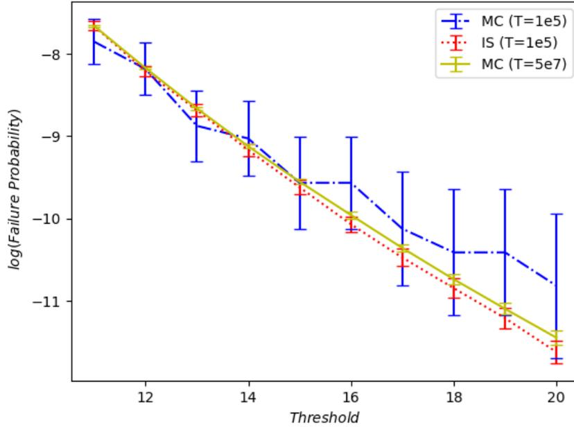
FIGURE 3.4: A comparison of the two MC estimates, and the IS estimate of  $p(b)$  for various  $b$  values in the case of  $f = \frac{1}{\epsilon}e_6$ .
