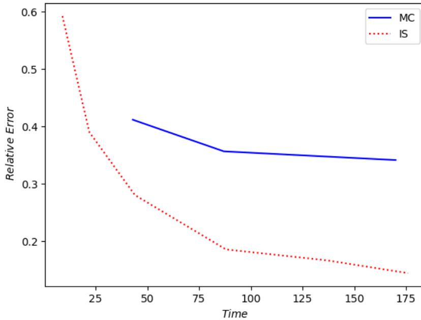
FIGURE 3.6: Comparison of computation time (in seconds) and the resulting error for MC and IS, in the case of  $f = \mathbf{1}$  and  $b = 15$ .
