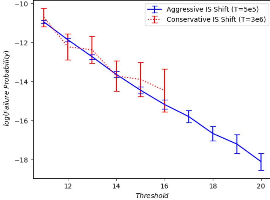
FIGURE 5.8: Comparison of IS methods for a uniform force. For the “aggressive” method, we choose a shift  $\tau = \ln(b)$  and perform  $5 \cdot 10^5$ , while the “conservative” method uses a smaller shift in accordance with the constants in Theorem 4.1.3 and  $3 \cdot 10^6$  trials.
