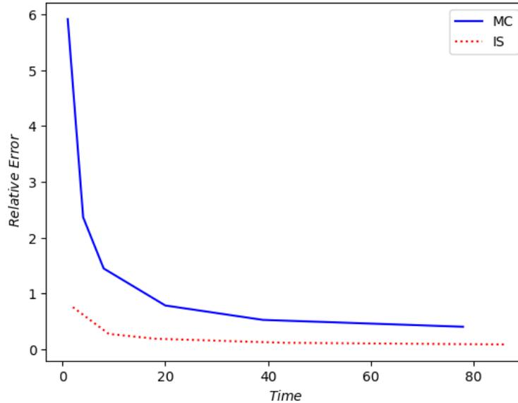
FIGURE 5.6: Amount of accuracy achieved for various computation times (in seconds) using both MC and IS algorithms. Here we take  $f = 10 \cdot \mathbf{1}$ ,  $b = 10$ .
