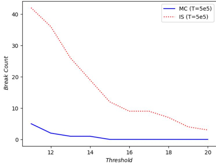
FIGURE 5.2: Comparison of the number of break events for Monte Carlo and importance sampling methods in 500,000 trials, for  $f = \frac{5}{\epsilon} e_6$ . In the IS algorithm, we use  $c = \frac{1}{5}$ .
