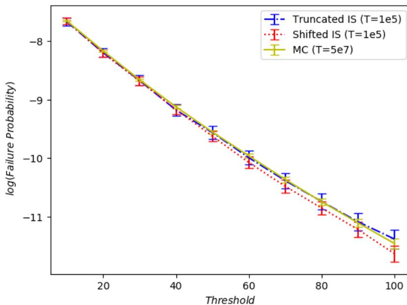
FIGURE 3.8: Comparison of different choices for the importance sampling measure  $Q$  for the case  $f = \frac{1}{\epsilon}e_6$  and 100,000 trials for each IS method. We can see that using a truncated normal distribution provides greater agreement with the “true” probability value obtained from a long MC simulation.
