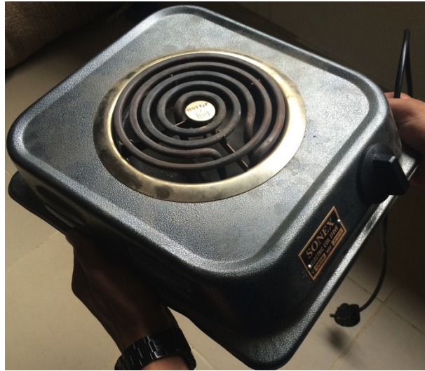
Figure 4: G-coil Electric Stove (Photographed during fieldwork, 2014)
