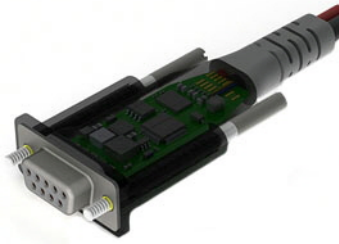
Figure 4: Rendering of circuit board in VGA cable from ISC Custom Cables and Electronic Inserts (ISC Custom Cables, 2019)
