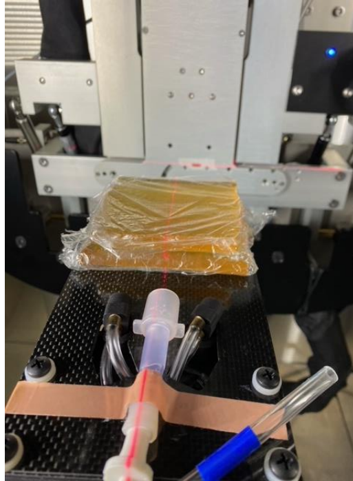
Figure 14: 2 cm Bolus phantom used for PDC verification (lasers set to isocenter).
