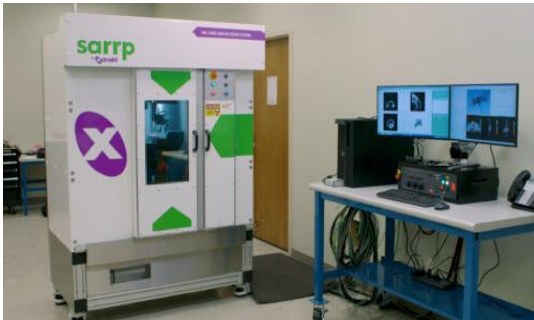
Figure 1: Xstrahl SARRP Pro System adjacent to remote X-Ray Controller (MP1) and SARRP control software [2].
