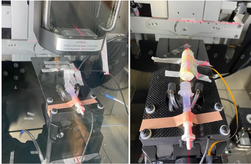
Figure 15: Calibration setup for MOSFET detectors using farmer chamber (left). PDC verification setup using MOSFET detectors inserted into mouse phantom as 1 cm depth (right).
