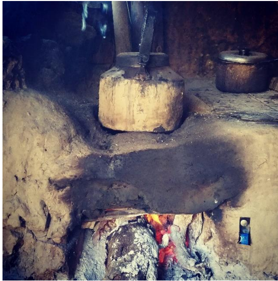
Figure 11. Stove Use Monitor (SUM) nailed to mud stove
