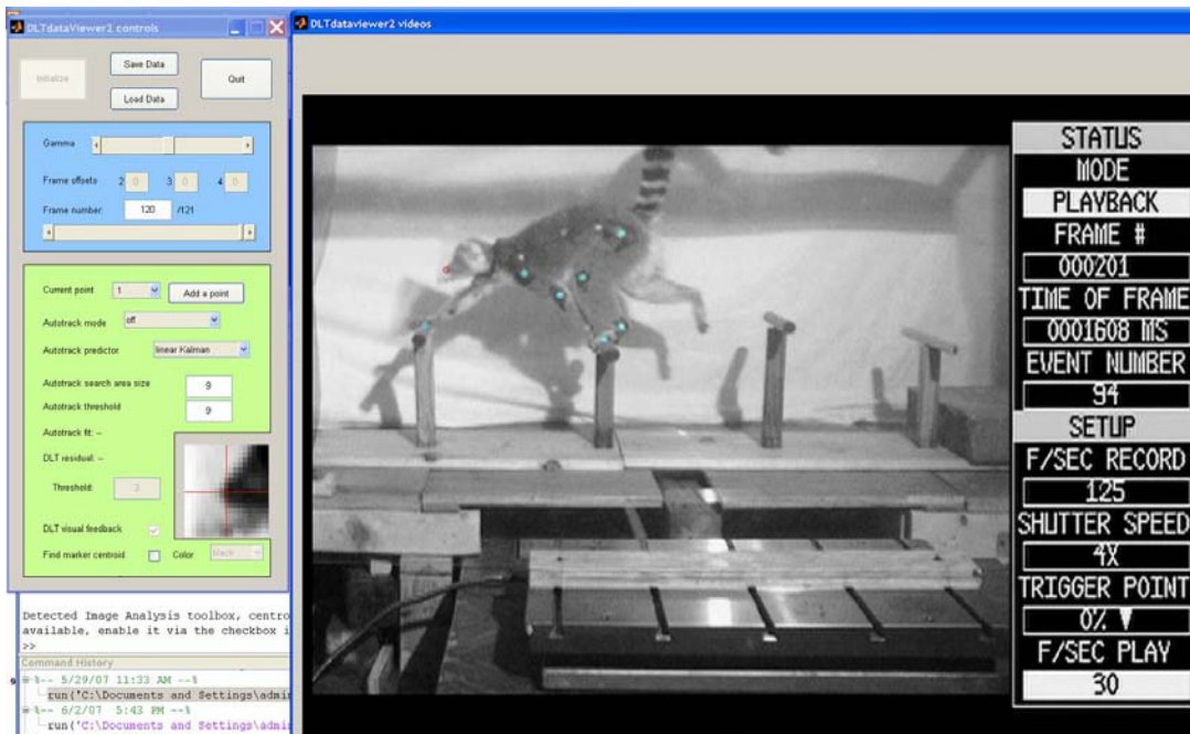
Figure 14: A single digitized frame in DLTdviewer. In the right window digitized points are displayed after direct placement from user input or automated tracking. In the left window, parameters for autotracking, point creation, and video navigation are available.
