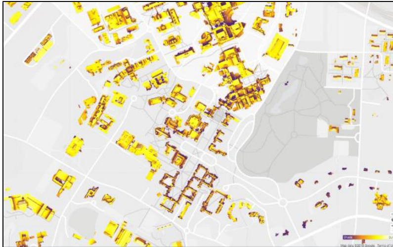
Figure 9. Shading effect parameters for Duke University are obtained from Google Project Sunroof database.
