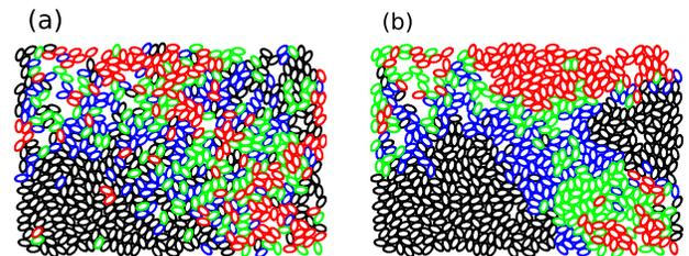
FIG. 4 (color online). Mobility of the particles (ellipses) in an arbitrary time. The packing fraction of the system is  $\phi = 0.932$ . The time delay  $\tau$  equals (a) 10 cycles and (b) 1000 cycles. The various colors represent particles with a similar mobility range. Specifically, the colors correspond to the following fractional changes relative to all the particles: red,  $0.90 \pm 0.1$ ; green,  $0.70 \pm 0.10$ ; blue,  $0.50 \pm 0.10$ ; and black,  $0.20 \pm 0.20$ .
