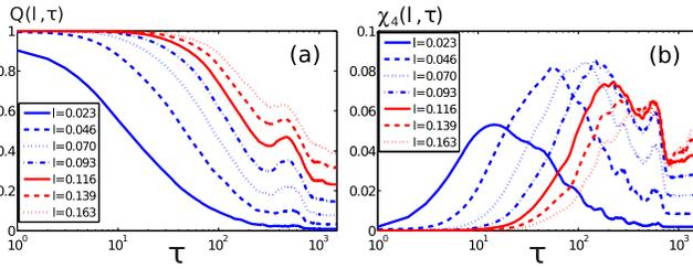
FIG. 5 (color online). (a)  $Q_s(\tau)$  and (b)  $\chi_4(\tau)$  for a system of isotropically compressed ellipses with a (highest) packing fraction of  $\phi = 0.916$ . The unit of length scale,  $l$ , is the semiminor axis of an ellipse.
