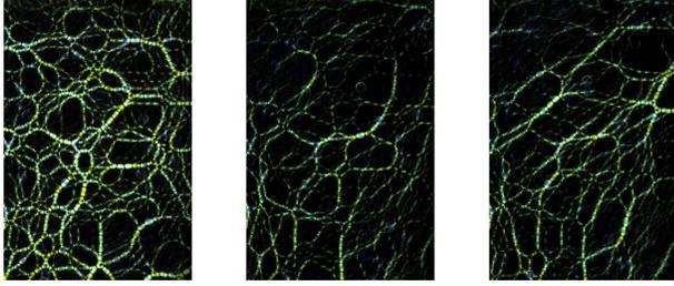
FIG. 2 (color online). Photoelastic images showing how the force network evolves over 999 cycles of cyclic compression, applied to a system of disks at  $\phi = 0.863$ . The cycle numbers of images from left to right are 1, 500, and 999.
