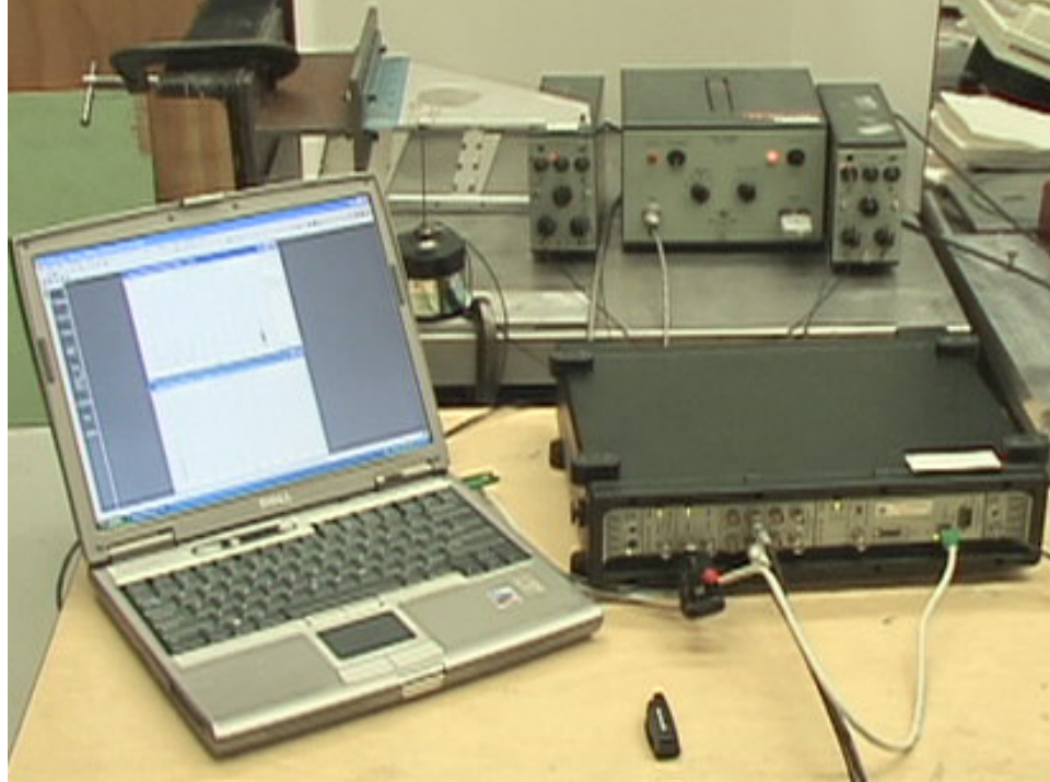
FIGURE 2.5: Equipment setup for vibration tests for determining the natural frequencies for the structural models
