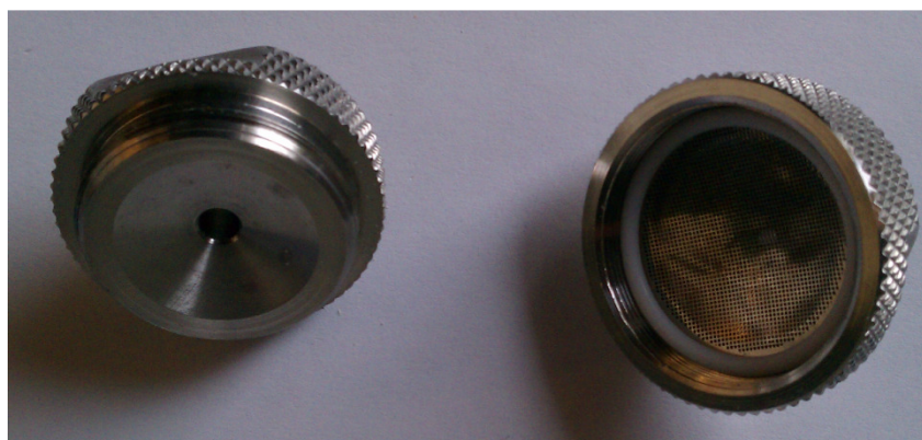
Figure 32. Re-usable syringe filter. (Top) Assembled. (Bottom) Disassembled.
