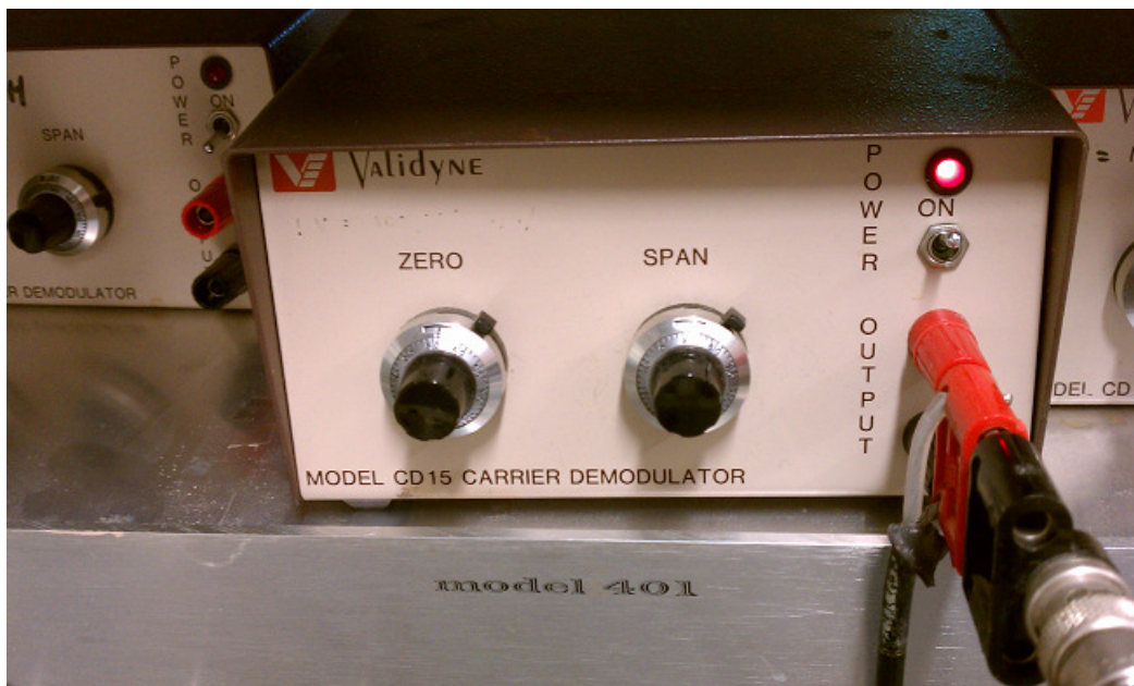
Figure 16. The signal from the pressure transducer is amplified using the Validyne Model CD15 Carrier Demodulator. The zero may be adjusted by using the knob on the left, and the gain by the knob on the right.
