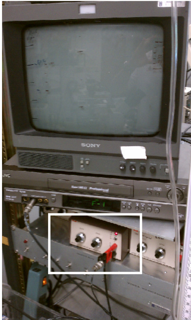
Figure 17 The signal from the pressure transducer is amplified (white box) before being input into the video recording unit (top of photograph). See Figure 17 for a close up view of the pressure transducer.
