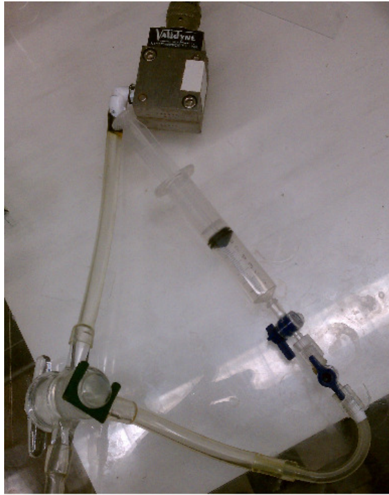
Figure 14. Syringe attached to the pressure transducer. Pressure is applied using the syringe. This pressure goes to both the micropipette and the pressure transducer, which converts the pressure into a voltage.
