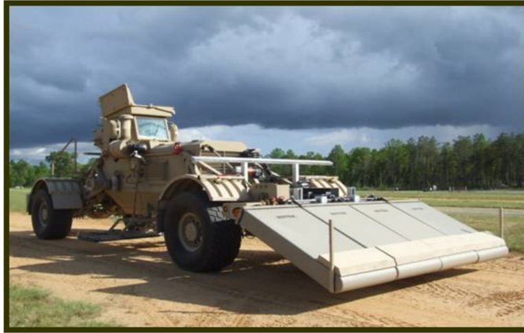
FIGURE 1.1: The NIITEK Husky Mounted Detection System (HMDS), which consists of 4 GPR antenna array panels (each with 12 channels) mounted in front of a Husky route clearance vehicle [14].
