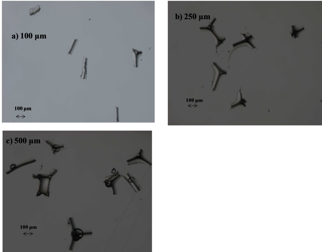
Figure 26: Microscopic imaging (60 time magnification) of fragmented foam with particle size a) < 100 \mu\text{m} , b) < 250 \mu\text{m} , and c) < 500 \mu\text{m} in series.
