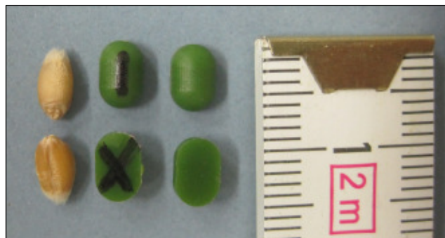
Figure 1. Comparison of simulated RFID markers with wheat grains used in these experiments.
