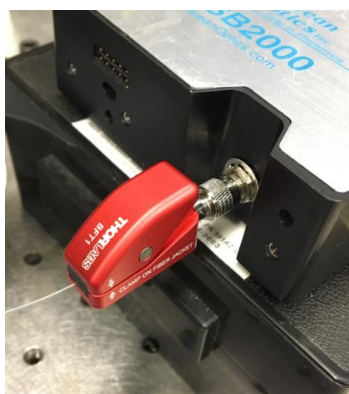
Figure 48: Bare fiber terminator used to fix the optical fiber and the spectrometer
