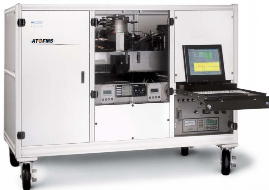
Figure 3: TSI ® Series 3800 Aerosol Time-of-Flight Mass Spectrometer [26]
