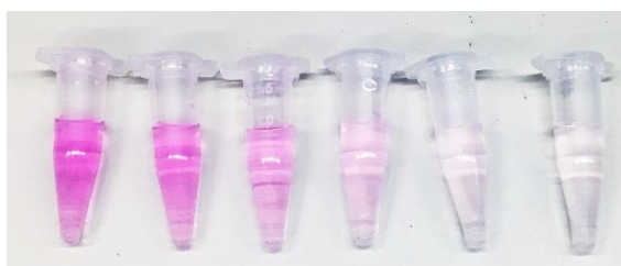
Figure 35: The colors of six different concentrations of nitrate are well developed
